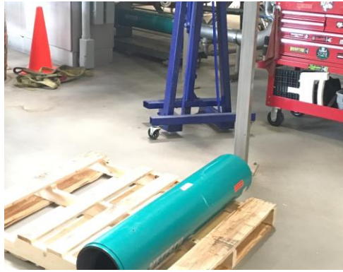
Rubber lined stator prepped for another quarterly replacement.
